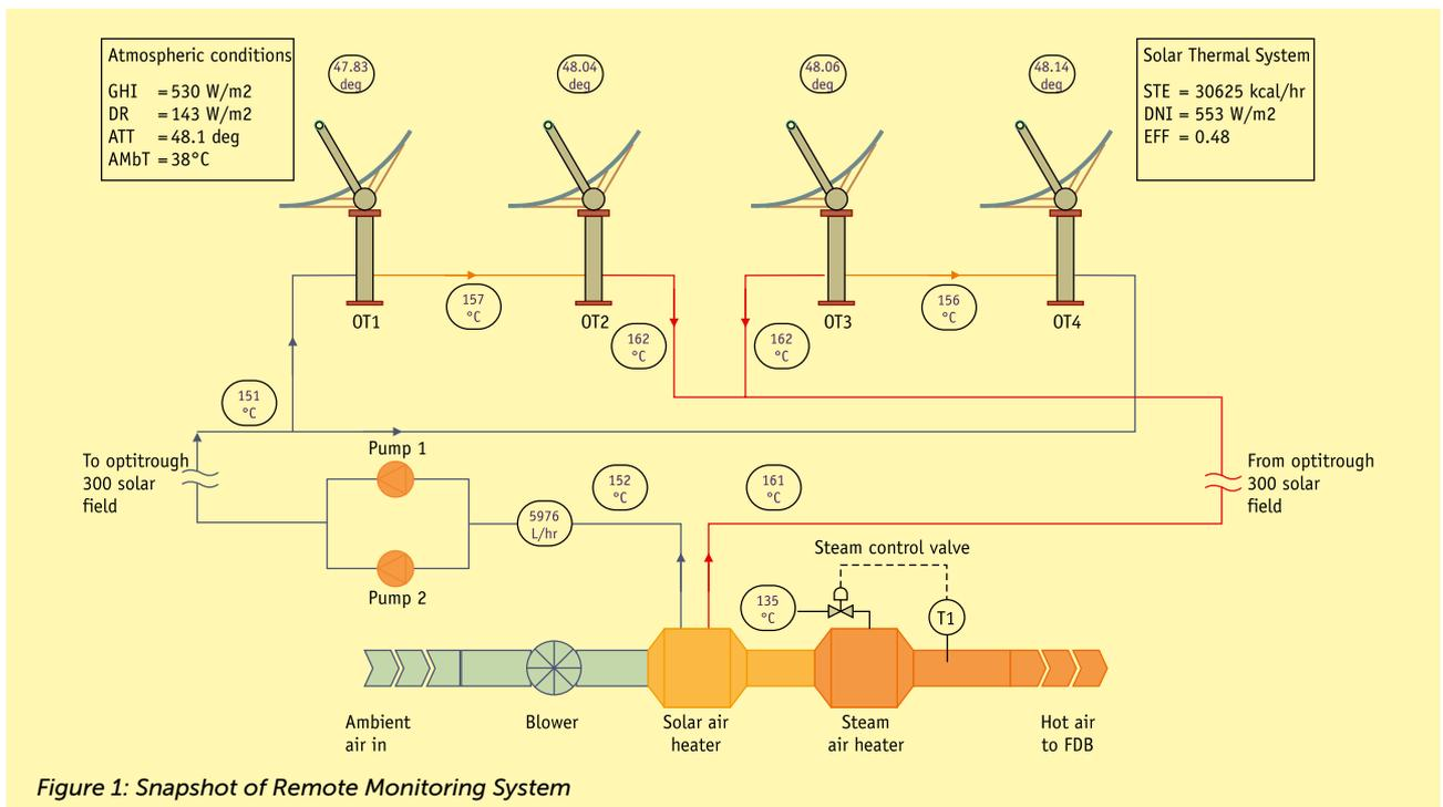
Figure 1: Snapshot of Remote Monitoring System
